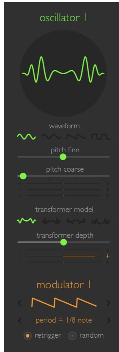
Oscillator waveform: sine, triangle, saw, square
